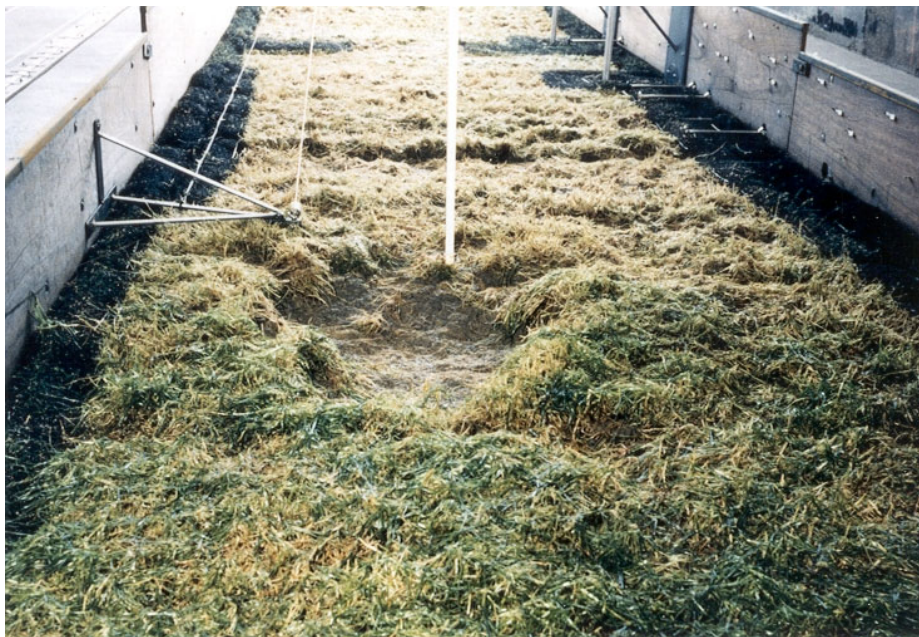
Figure 3.5 Erosion hole after 11 hours of wave attack during large scale test with the turf from the seadike (Source: Delft Hydraulics)
