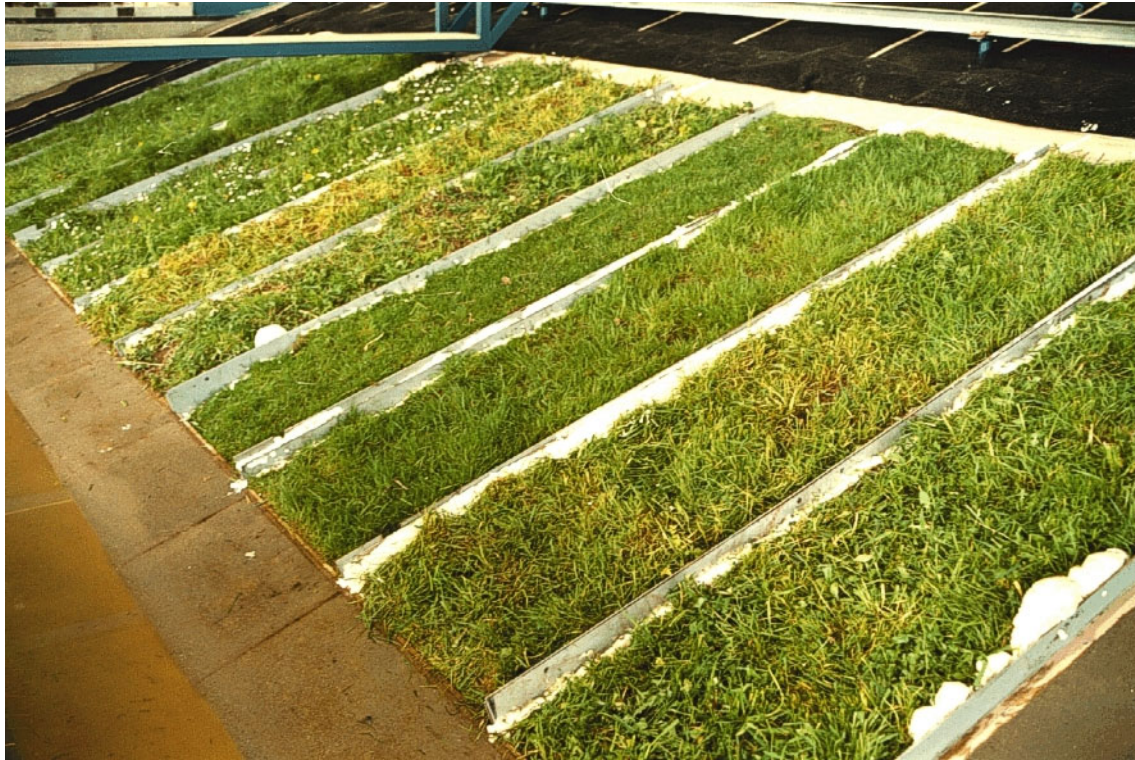
Figure 3.4 Large scale tests on the turf from the riverdikes (Source: Delft Hydraulics)
