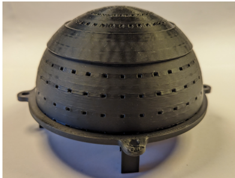
(b) Big Diamond PUF: Cap closed, con sealing the device. Currently without any resin
