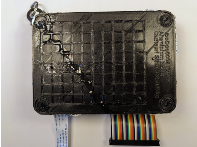
(b) Front view of the PUF enclosure when closed, filled with epoxy. Note the drilling hole on the left center (further discussed in Section 3.7).
