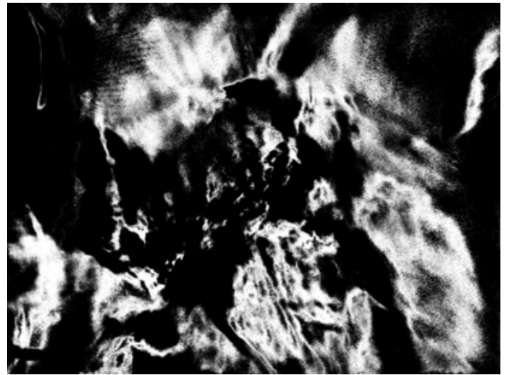
(b) Image displaying invalid Sections (white) of Figure 4.5.1a that could not be error corrected using binning (amounts for over 80%).
