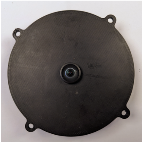
(a) Big Diamond PUF: 180° camera lens placed into the open enclosure. With the camera sensor underneath.
