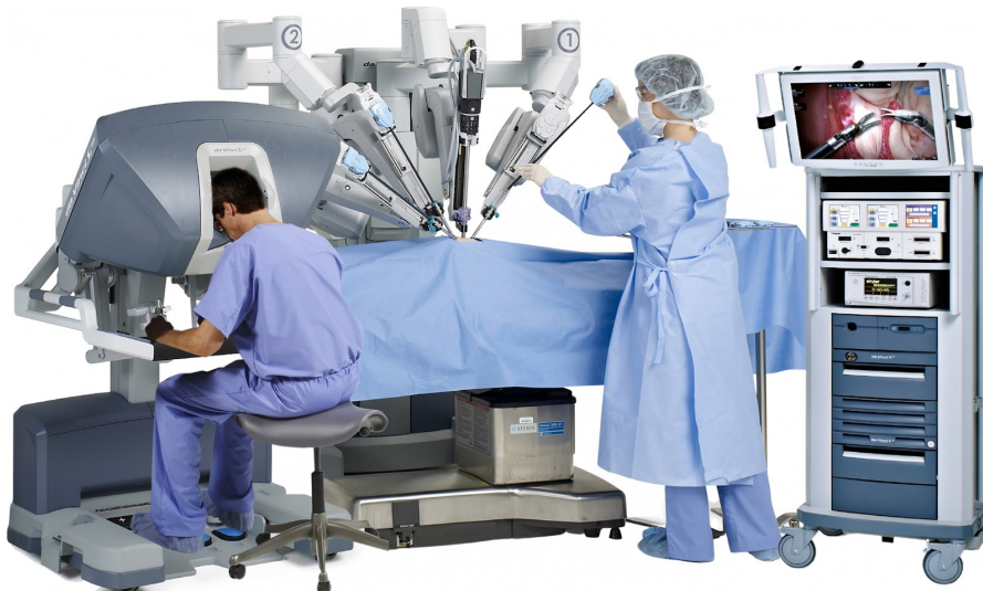
Figure 2.1: Example of a "no delay" teleoperation robot, the Da Vinci surgery robot picture from cghmc
