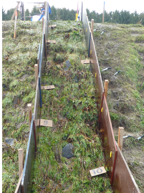
(a) Overflow test section after final test ( t = 12:00 h, q_{max} = 165 l/m/s)
