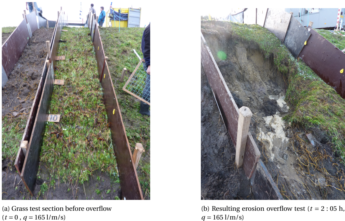
Figure 3.14: Headcut formation through grass due to constant overflow tests at the Wijmeerspolder
