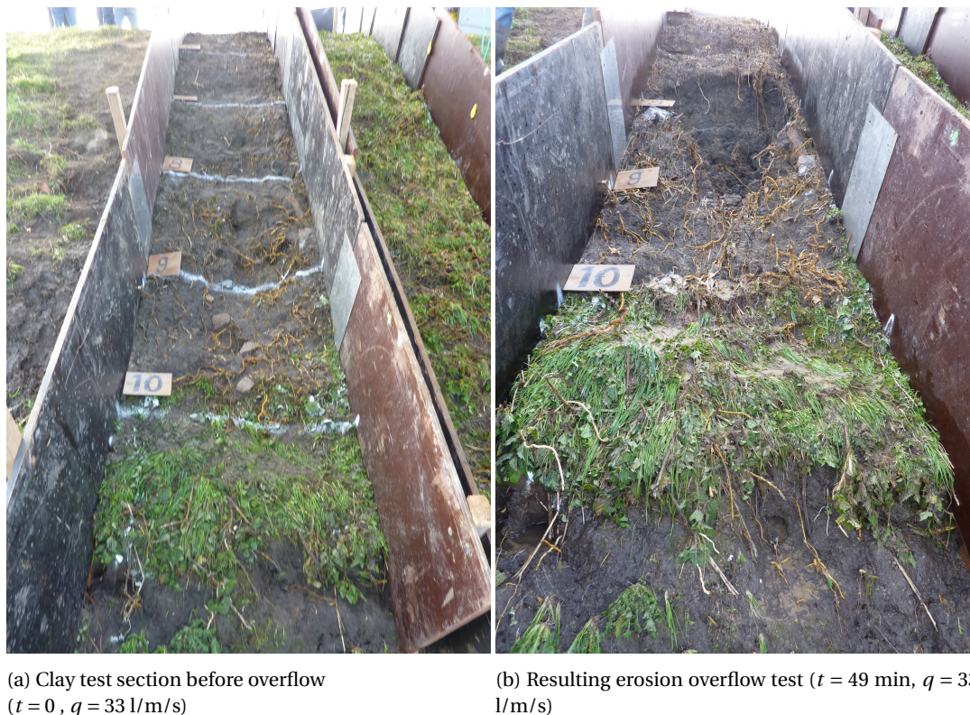
Figure 3.13: Headcut formation in clay due to constant overflow tests at the Wijmeerspolder
