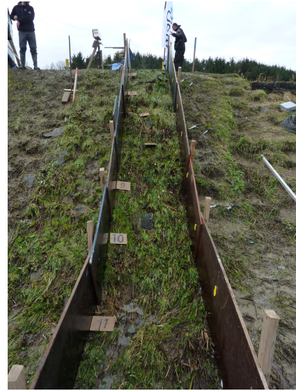
(b) Overflow test section after fifth test ( t = 10:00 h, q_{max} = 125 l/m/s)
