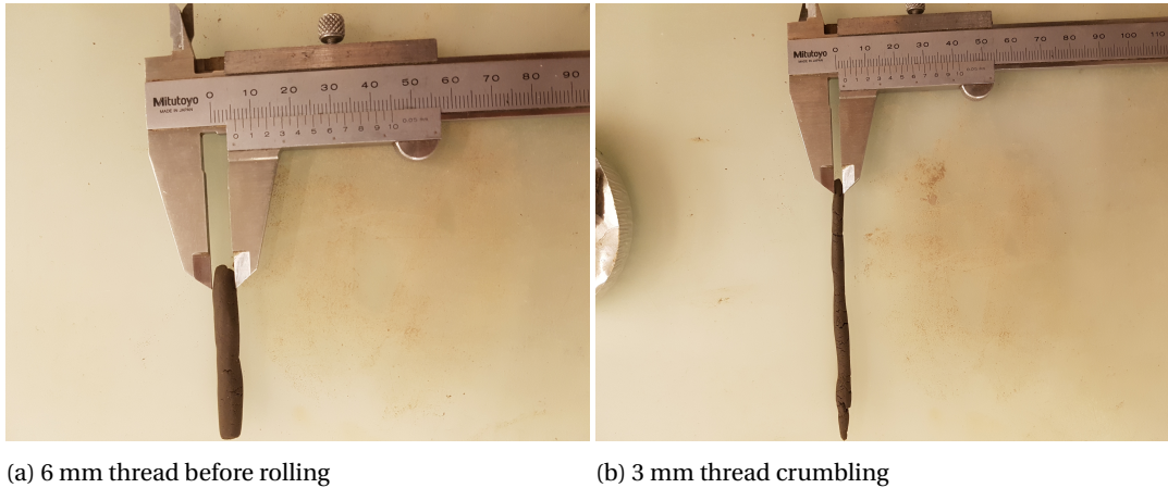
Figure A.10: Execution of the Plastic limit test
