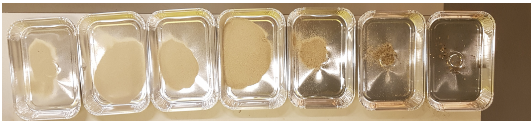
Figure A.4: Separated grain sizes from fine to coarse
