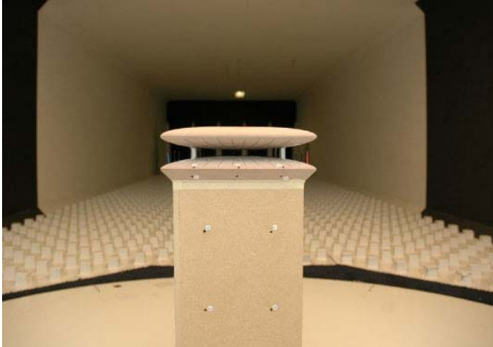
Figure 26.1: 'venturi' roof design by Bronsema in E,W&F research in the wind tunnel at Peutz in Mook.
