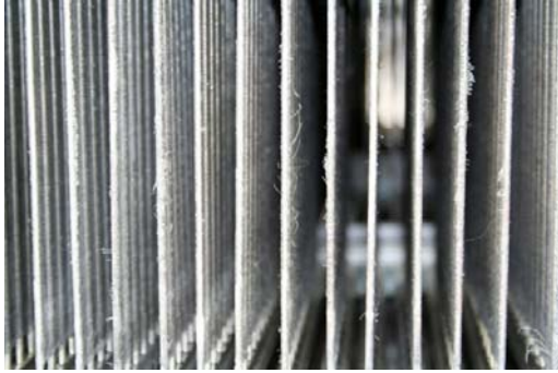
Figure 21.4: Side view of the woven copper wire mats in a linear heat exchanger
