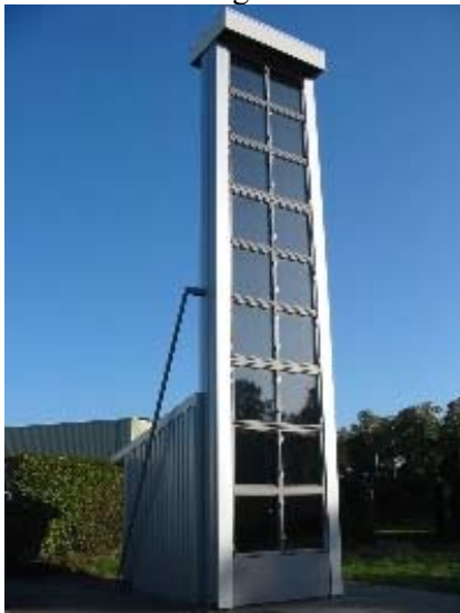
Figure 10.1: Mock-up of solar chimney in the E,W&F research. project at Peutz in Mook
