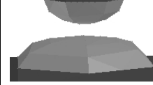
Figure 11.2c: The roof parts are stretched in the vertical direction. The roof plate is not changed. Both ellipsoids are 4.8 m high and the separation is 2.5 m, so the contraction ratio is 0.2.
