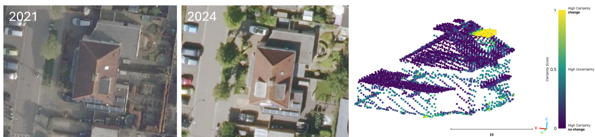
Figure D.1.: Change detection results for a building where a dormer was added between the national height model of the Netherlands number 4 (AHN4) (reference point cloud dataset) and national height model of the Netherlands number 5 (AHN5) (target point cloud dataset) epochs. The added structure is identified with high certainty in change. Orthophotos from 2021 and 2024 are provided for context, source: Beeldmateriaal Nederland .
