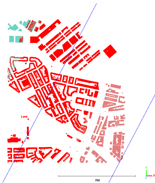
(a) Simulated scene (top view), showing all three flightstrips (light blue, red and pink). Dark blue represents the flightlines.
