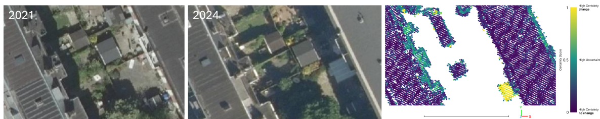
Figure D.2.: Detection of a lateral extension to a building structure, constructed between AHN4 and AHN5 epochs. The newly added portion is highlighted with high certainty of change. Orthophotos support the structural modification, source: Beeldmateriaal Nederland .
