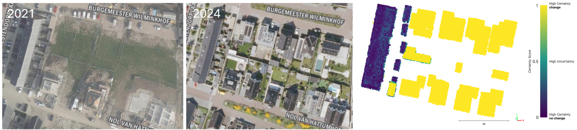
Figure D.6.: Newly constructed buildings are identified between AHN4 (reference point cloud dataset) and AHN5 (target point cloud dataset) point clouds. The detection algorithm assigns high change probability values to the new structures. Orthophotos from 2021 and 2024 are provided for context, source: Beeldmateriaal Nederland .
