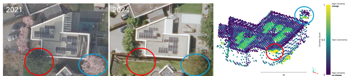
Figure D.4.: False change detection due to tree points within building-labelled raster cells (blue circle). In addition, removed opaque vegetation between epochs results in regions consistently labelled as changed due to persistent occlusion in the reference point cloud dataset (red circle). Orthophotos from 2021 and 2024 are provided for context, source: Beeldmateriaal Nederland.
