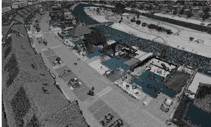
(a) AHN4. Several houses are poorly captured. Darker colors represent lower intensity values.
