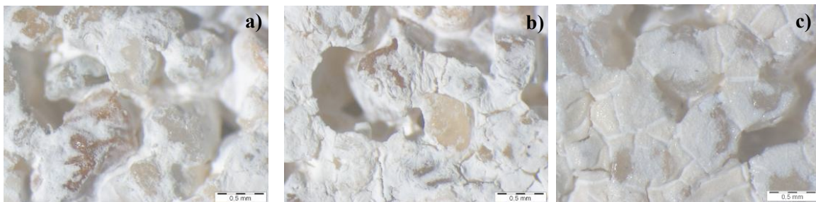
Fig. 2 – Stereozoom microphotographs (20x and 40x): a) Untreated specimen (arrows); b) Specimen treated with NLSE; c) Specimen treated with NS.
