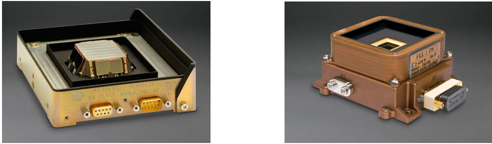
Figure 5.2: Bradford pyramid and four-quadrant Sun sensors. 2
