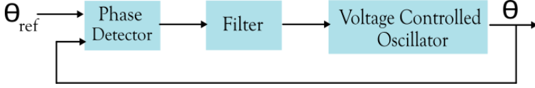
Figure 3.4 Block diagram of Phase locked loop system
