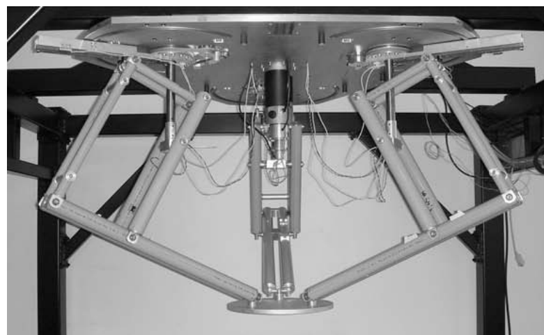
Figure 14. The PAMINSA manipulator [101].
