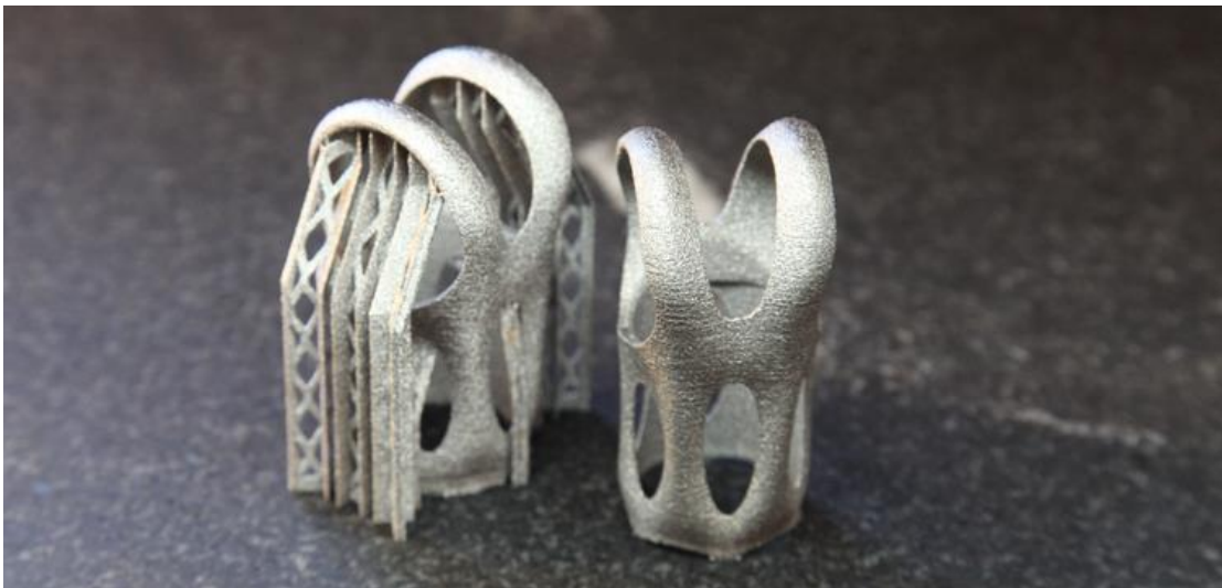
Figure 3-13 Parts made by EBM process ( http://pencerw.com )
