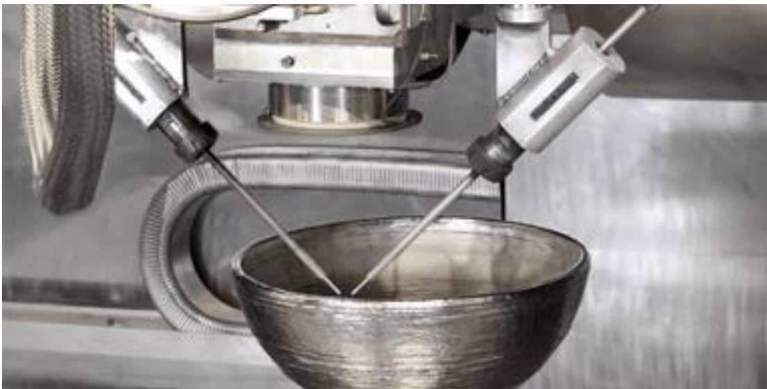
Figure 3-9 EBAM system from Sciaky ( http://www.sciaky.com/ )
