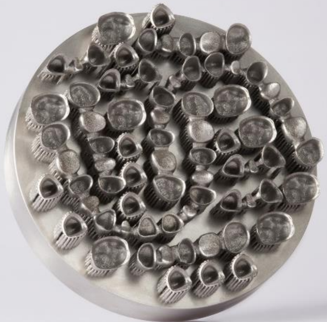
Figure 3-14 Sample Application from the Dental Industry on a EOS M 100 Building Platform ( http://www.eos.info/dental )
