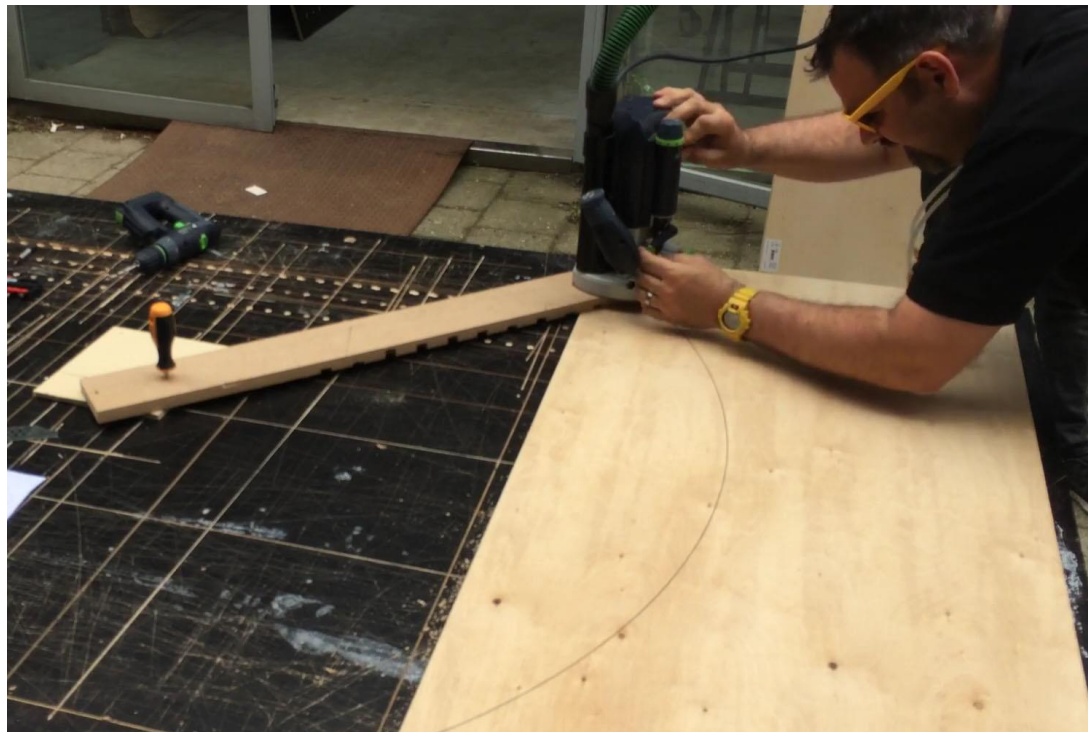
Figure 5-45 A router is fixed to a specific radius to cut the plywood
