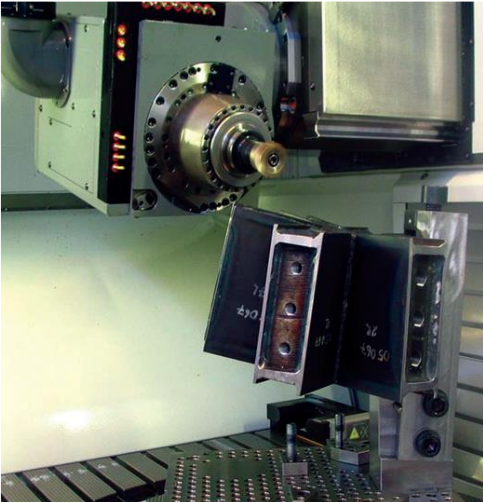
Figure 4-12 Machining of nodes for final accuracy (Knippers & Helbig, 2009)
