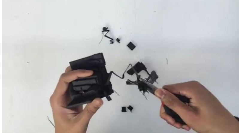
Figure 5-51 Removal of the scaffolding structure
