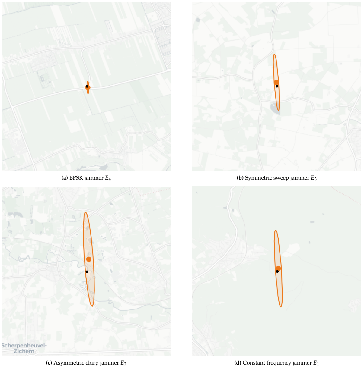
Figure 3.18: Final geolocation estimates for Scenario 1. The true emitter geolocation is shown as a black dot, the estimated geolocation as an orange dot, and the 95% confidence ellipse in orange.
