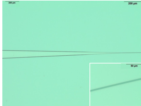
Figure 5.13: Microscopic image of SU-8 waveguide with tapers
