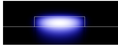
Figure 4.3: Fundamental mode in the two dimensional waveguide
