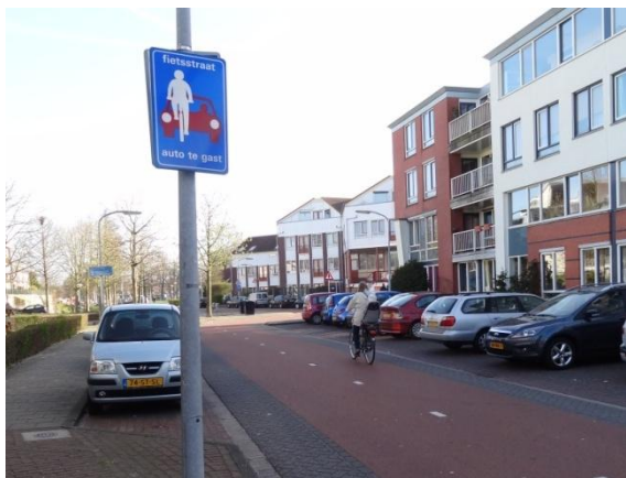
FIGURE 23: BICYCLE STREET WITH LANE LINES IN THE MIDDLE OF THE STREET AND A BLUE TRAFFIC SIGN. THIS BICYCLE STREET DIFFERS FROM OTHER SINGLE-LANE BICYCLE STREETS, BECAUSE ON THIS BICYCLE STREET A LANE LINE HAS BEEN APPLIED.
