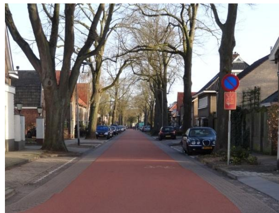
FIGURE 24: BICYCLE STREET WITHOUT LANE LINES AND WITH A RED TRAFFIC SIGN. THIS BICYCLE STREET DIFFERS FROM OTHER SINGLE-LANE BICYCLE STREETS, BECAUSE HERE A SUBSTANDARD TRAFFIC SIGN HAS BEEN APPLIED.
