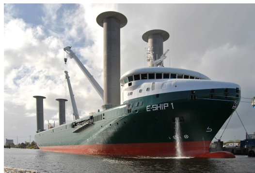
Figure 2. "E-Ship 1" of Enercon equipped with Flettner rotors (picture by Carschten).
