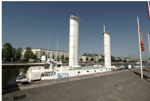
Figure 2. “Alcyone” of Cousteau equipped with Turbosails (picture by Entomolo).
