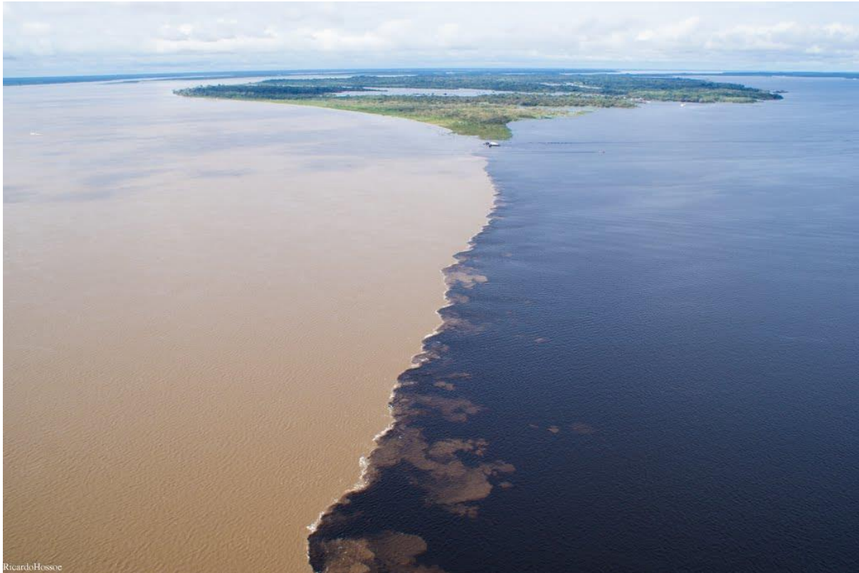
Figure 41 Photograph of the Meeting of the waters, the merging of the Solimões (right) and the Rio Negro (left), showing floating foam around the shear layer and flow instabilities below the water surface. Source: http://www.panoramio.com/photo/90000345
