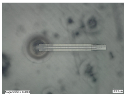
Optical microscope image to check printed cantilever.
