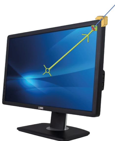
Figure A.9: Screen corner clamp, used as a quick and dirty way to align the apertures of the fluid interface to the 2PP writing field. The cross-hair could be positioned on the camerafeed window at the location of the centre of the writing field. The spring-loaded clamp could easily be attached and removed.
