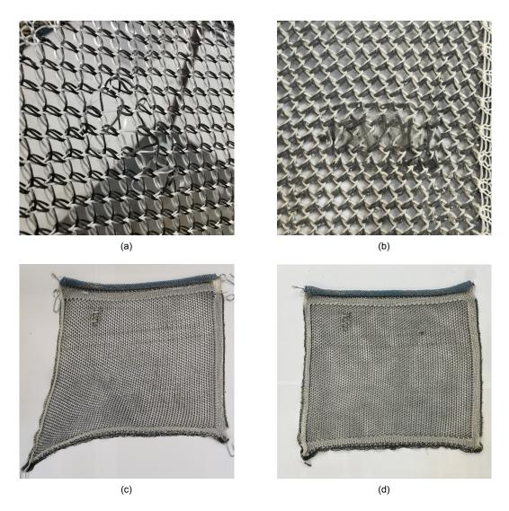
Figure 4.11: Fabric reuse: (a) initial defect, (b) defect after the fabrication of six prototypes, (c) deformed fabric after casting four identical prototypes, (d) fabric after tensioning it back into its original shape
