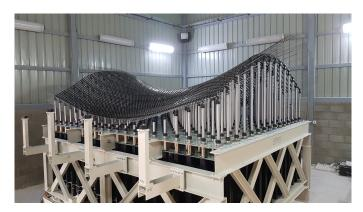
Figure 2.5: Example of an adaptive mold system: Adapa Adaptive Mould D200 [1]
