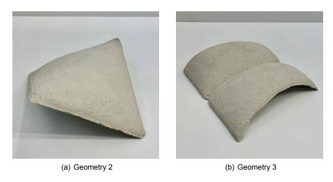
Figure 4.10: Finished prototypes of prototyping iteration 3: (a) Geometry 2 and (b) Geometry 3
