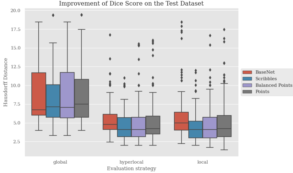
Figure 5.2: Hausdorff distances for the three methods that are being compared in this paper. Lower is better.
