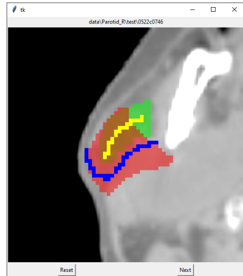
Figure 4.2: Screenshot of the application used to annotate the test set. Green represents an undersegmentation, red an oversegmentation and orange a correct segmentation. The fore and background scribbles are shown in yellow and blue respectively.
