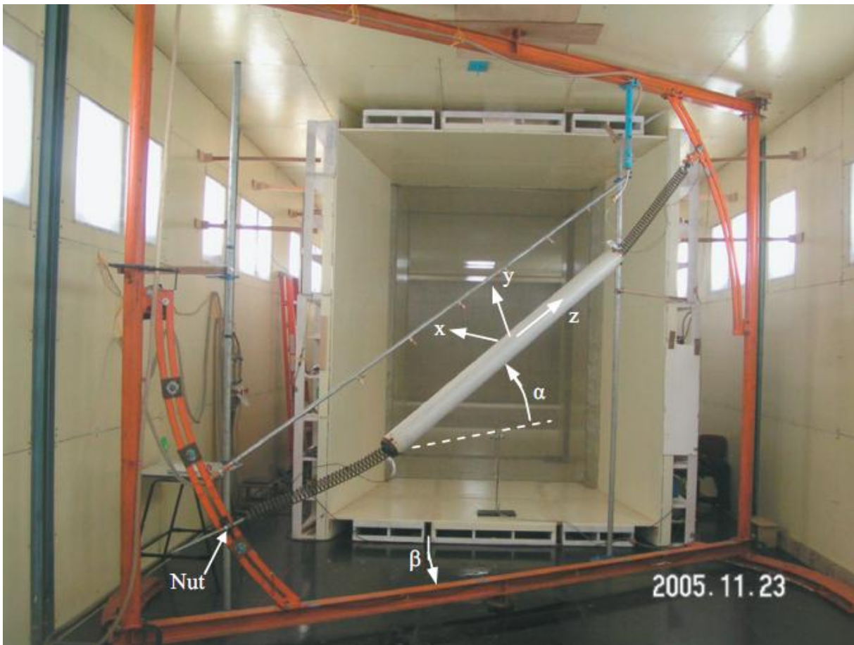
Figure 9.3: New setup for wind-rain-induced cable vibration of [19].
