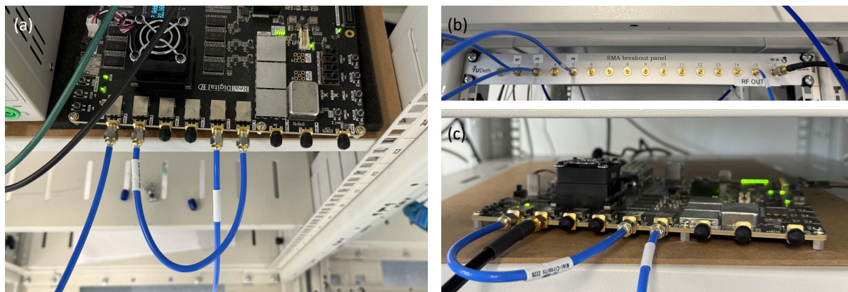
Figure 5.2: The RFSoc 4x2 board setup. (a) shows the loopback connection for validating the signal generation and acquisition. (c) shows the same DAC and ADC connected to the cryostat cabling via the breakout panel in (b)
