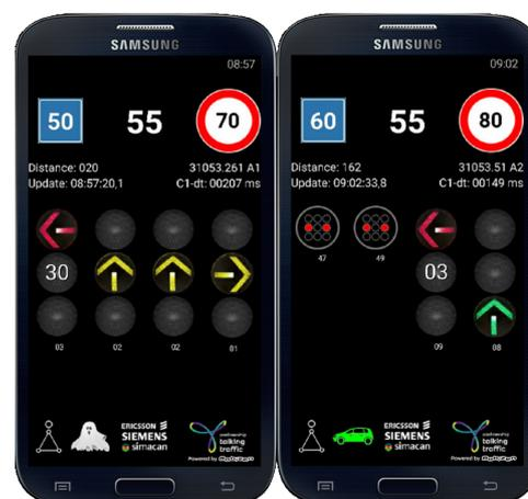
Figure 3.14: Priotalker app developed by Siemens to inform arriving vehicle. The advisory speed is given top left in blue. The signal states of the oncoming TLC is shown in the middle with the expected time until a switch when that is available.
