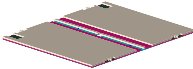
Figure 4.12: Characterisation Fixture without the GSG pads. Only the TL is shown; Pads are not shown here as ADS 3D view ran out of memory to process the structure with pads.
