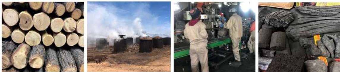
Figure 7: Production of charcoal using kilns from encroacher bushes.
