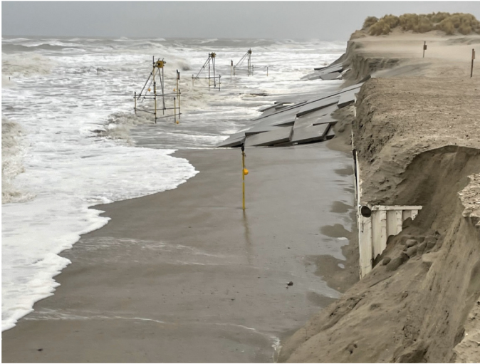
Fig. 7. The setup at 1 January 2025, the onset of high tide of storm 3. The cliff location and beach elevation are mostly uniform alongshore.
