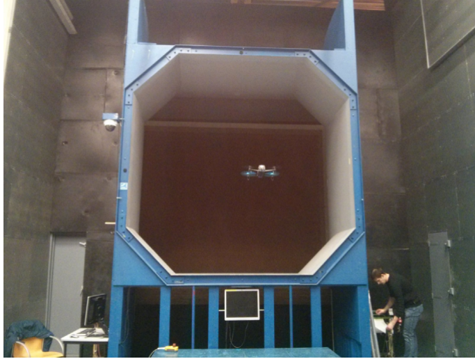
Figure 1.7: A quadrotor flying in a open jet wind-tunnel [57]
