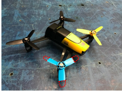
Figure 1.2: Example of a quadrotor with partial rotor failure due to blade damage (red-dash line).
