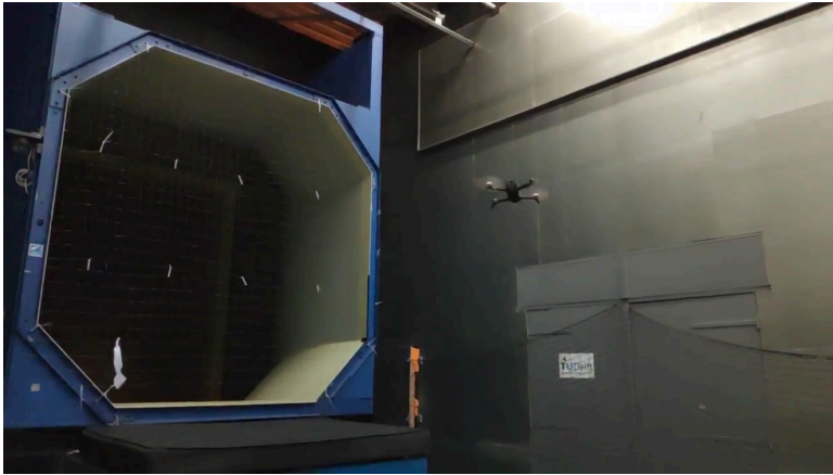
Figure 5.12: Snapshot of the tested quadrotor in the wind tunnel, with removal of rotor 1 and 3.
