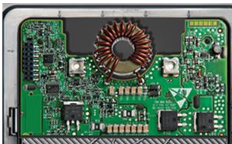
Figure 1.12: Example of power optimizer.[19]
