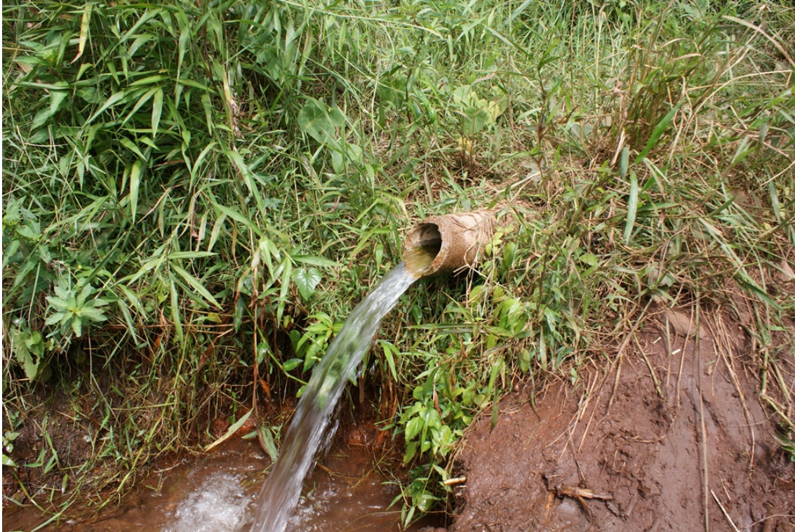
Figure A.26: Groundwater outflow in Godi catchment (measurement location Godi_3). This concerns groundwater. pH, EC and Temperature values also indicate that this water is not similar to the water flowing on top of it (small irrigation canal). The pipe is only placed to guide the water. (March 2014)
