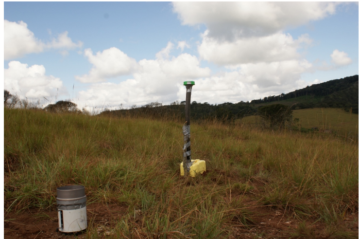
Figure C.2: Rain gauge and tipping bucket installed at the top of the Inselberg
