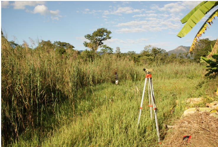
Figure E34: Measuring cross sections along and perpendicular to the river Ruaga
