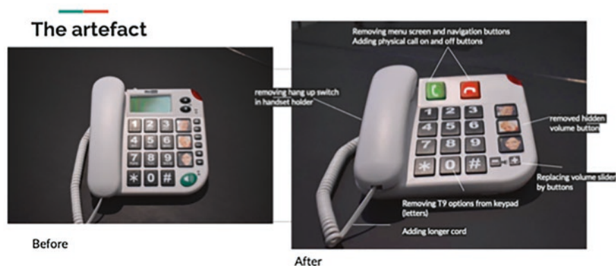
Image 16.6 Picture memory phone before and after modifications
