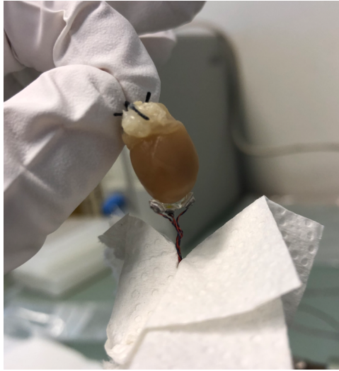
Figure 3.24: Fitting of the apex-cup device to the ex-vivo setup of rat heart ventricular epicardium
