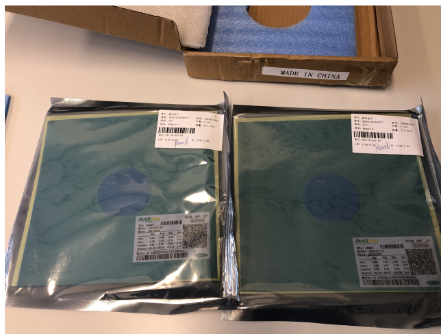
Figure 6.1: The mini-LED wafers used in the system, in flip-chip packaging on carrier films
