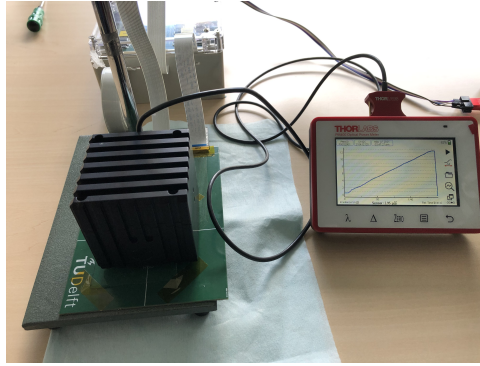
Figure 5.30: Setup for calibrating the irradiance settings in the user interface program
