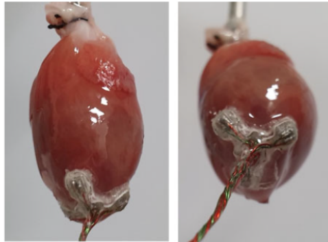
Figure 3.12: The apex-cup device is glued to the rat's ventricular apex
