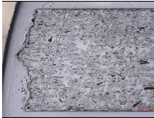
Figure 82: Pristine Composite Tensile Test Fracture Surface
