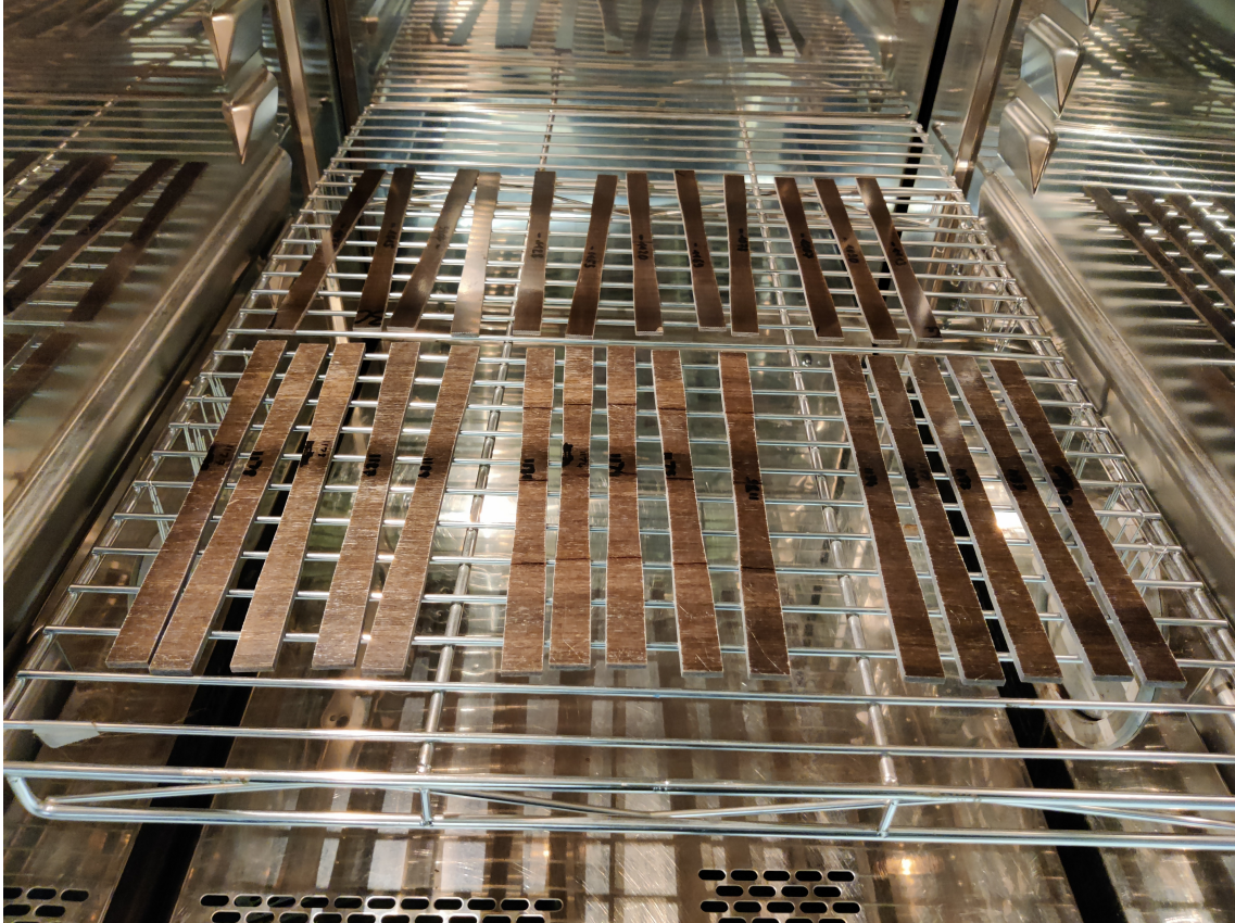
Figure 37: Hygrothermal Aging of the Transverse Flax Composites
