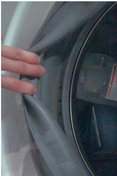
Figure 4.11 Degraded inner seal of used washing machine
