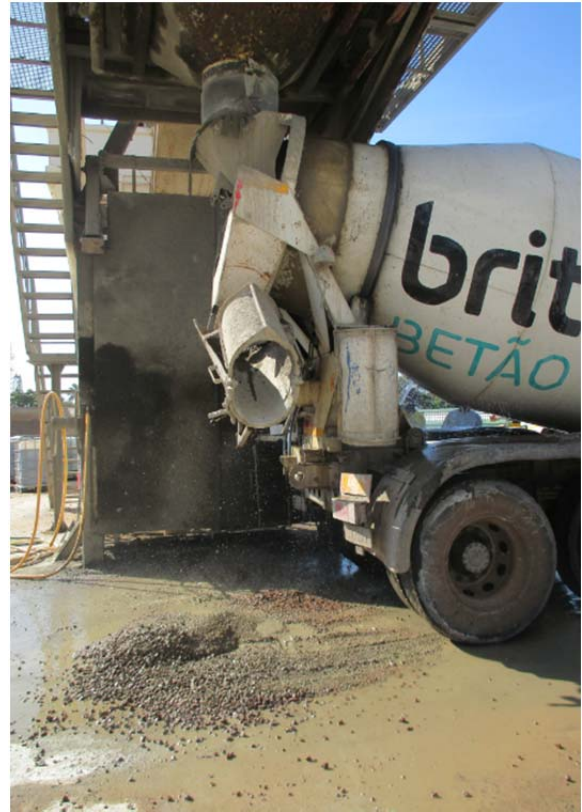
Figure 8.29 Filling-up the truck with ready-mix concrete (The excess water drops down from a side outlet)
