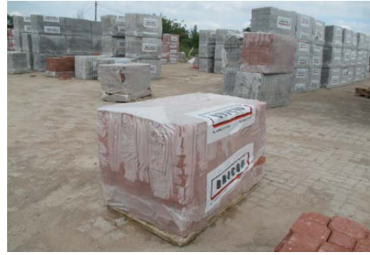
Figure 8.40 Curing with plastic wrap (saving water)
