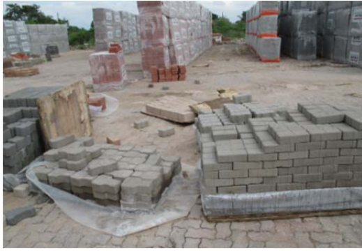
Figure 8.38 Freshly-hardened concrete blocks
