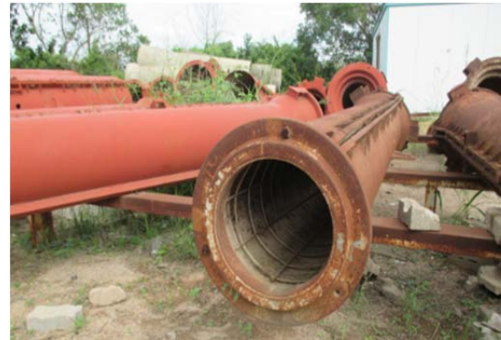
Figure 8.41 Formwork of reinforced concrete pipe
