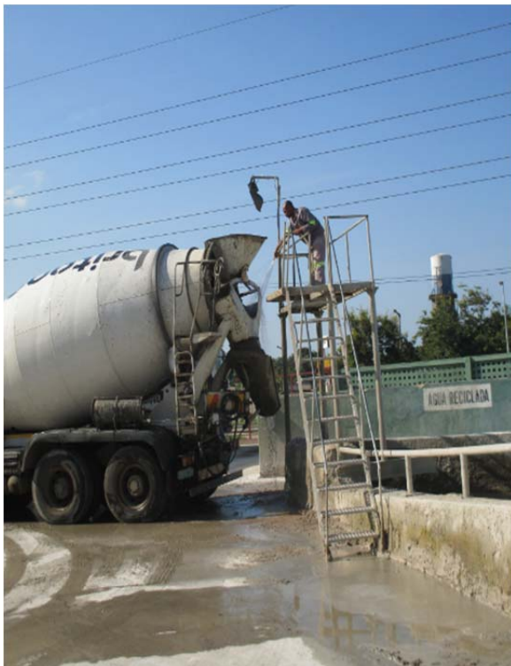
Figure 8.28 Washing the trucks (The floor is sloped to let the water flow into the recycling system)
