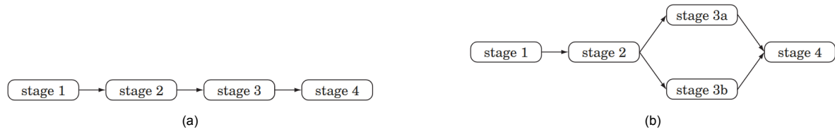
Figure 4.5: Example pipelines illustrations from [78, p.106]. (a) Linear pipeline: sequential chain of stages. (b) Nonlinear pipeline: data may be split to form parallel stages that perform the same operation. Introduces data parallelism for load balancing.
