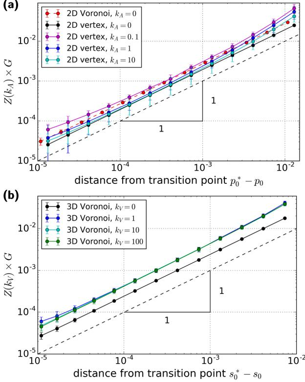
FIG. S2. For  $\gamma = 0$  and  $\ell_0 < \ell_0^*$ , the shear modulus  $G$  scales linearly with the distance  $\ell_0^* - \ell_0$  to the transition point (cf. Eq. (S39)). (a) 2D Voronoi and 2D vertex model, (b) 3D Voronoi model. Rescaling the shear modulus by  $Z$  defined in Eq. (S34) largely collapses the data for all  $k_A > 0$  values of a given model.
