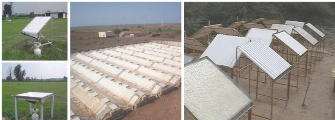
Fig.14 State of the art in radiative condensers
