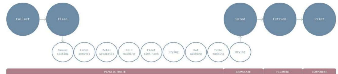
Fig.151: Recycled plastic filament's production process
