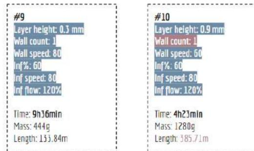
Fig.118: Final printing settings based on nozzle diameter
