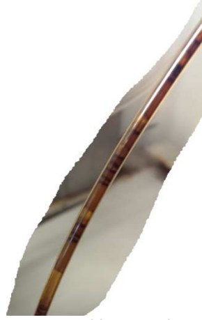
Figure 13: Fluids at the outlet of the core; appearing more like an emulsion than a foam.
