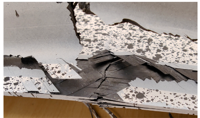
Fig. 16. Skin fracture of panel 2.
