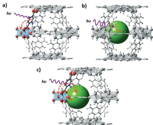
**Fig. 3** Different approaches to induce photocatalytic activity in a MOF scaffold: a) the organic linker is used as an antenna for light sensitizing and charge transfer to the inorganic cluster occurs; b) the MOF is used as a container for the encapsulation of a photocatalyst that directly absorbs light and c) charge transfer occurs between the MOF scaffold and the encapsulated catalyst.
