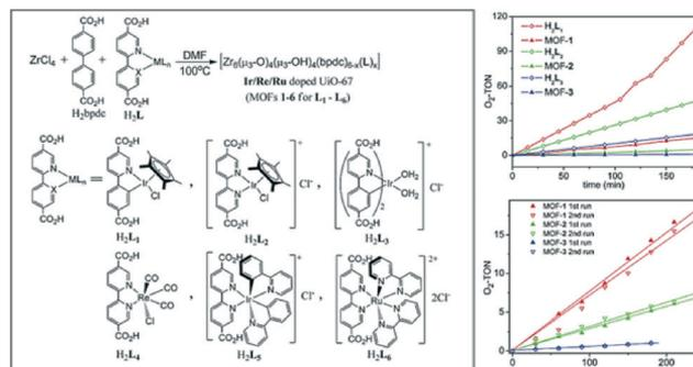
**Fig. 5** Doping of UiO-67(Zr) frameworks with molecular catalysts: schematic view (left), plots of O<sub>2</sub> evolving turnover number (O<sub>2</sub>-TON) vs. time for doped MOFs and the corresponding homogeneous analogues (top right), and recyclability studies (bottom right).<sup>71</sup> Reproduced with permission from the American Chemical Society.
