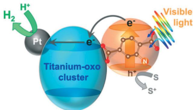
**Fig. 4** A schematic illustration of photocatalytic hydrogen production reaction over Pt-supported Ti-MOF-NH<sub>2</sub> on the basis of the LCCT mechanism.<sup>60</sup> Reproduced with permission from the American Chemical Society.
