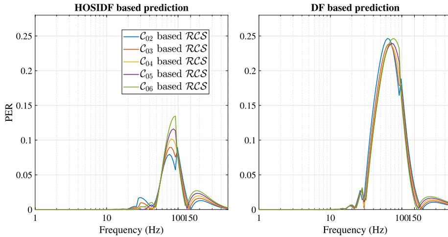
Fig. 22. Prediction error ratio plots of  $C_{02}$  to  $C_{06}$  based systems for input  $d$  based on  $L^\infty$  norm for the existing DF based and novel HOSIDF based methods. All systems have same  $|L_1|$  and PM.
