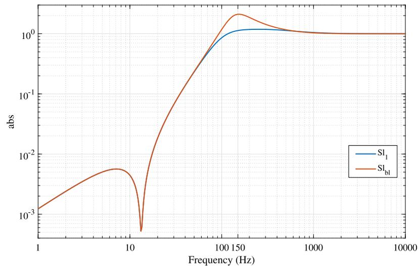
Fig. 25. Sensitivity plots  $S_{I_1}$  as defined by (21) and  $S_{I_{bl}}$  as defined by (23) for  $C_{02}$  based  $RCS$ .
