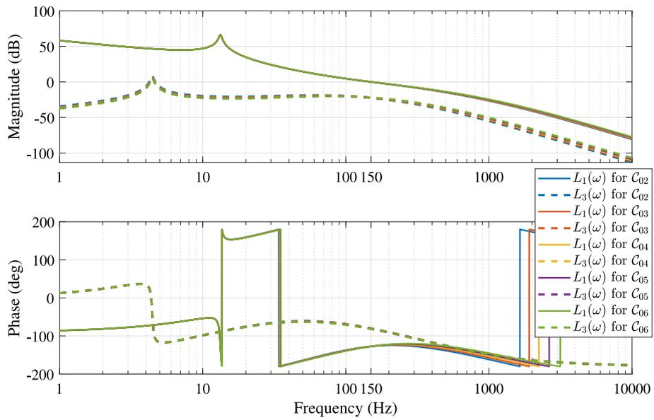
Fig. 14.  $L_1(\omega)$  and  $L_3(\omega)$  plots for five  $\mathcal{R}_{C_{gLP}}$  controller (refer (47)) based RCS.  $C_{02}$  to  $C_{06}$  based systems provide same phase lead  $\phi_{C_{gLP}}$  of  $20^\circ$  and same overall PM of  $50^\circ$ , but with different values of  $\gamma$ .
