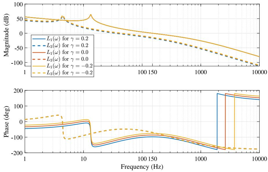
Fig. 12.  $L_1(\omega)$  and  $L_3(\omega)$  plots for three  $\mathcal{R}_{CI}$  controller (refer (45)) based RCS with  $\gamma = \{0.2, 0.0, -0.2\}$ .
