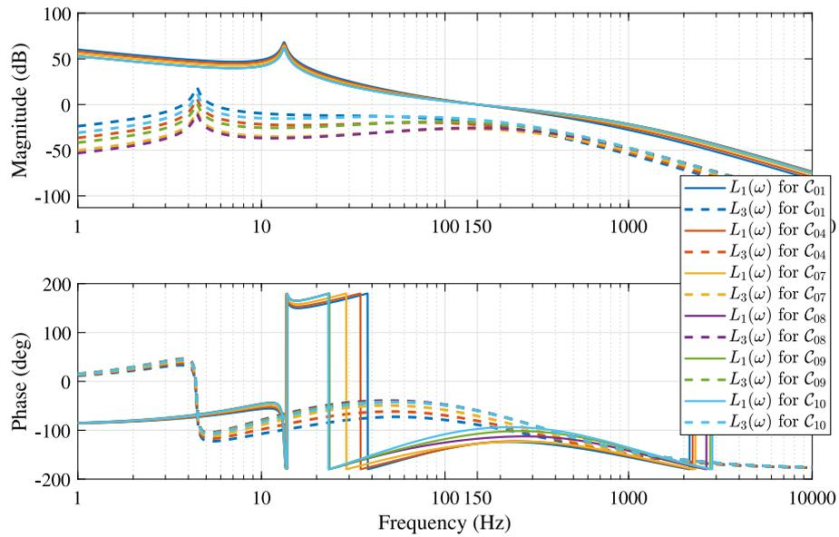
Fig. 15.  $L_1(\omega)$  and  $L_3(\omega)$  plots for six  $\mathcal{R}_{C_{gLP}}$  controllers (refer (47)) based RCS.  $\{C_{01}, C_{04}, C_{07}\}$  based systems have same PM with different  $\phi_{C_{gLP}}$ , while each group  $\{C_{01}, C_{10}\}$ ,  $\{C_{04}, C_{09}\}$ ,  $\{C_{07}, C_{08}\}$  based system provides same  $\phi_{C_{gLP}}$  but different PM. All controllers have same value of  $\gamma = 0.0$ .
