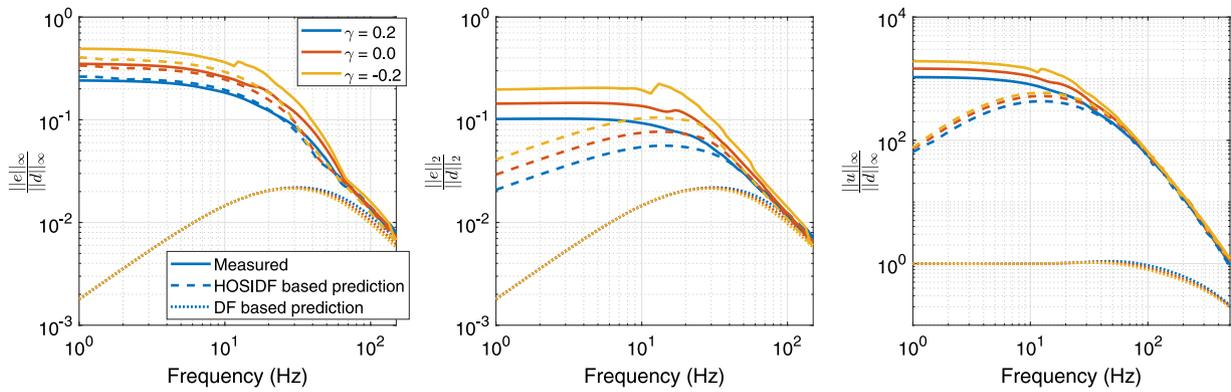
Fig. 17. Process sensitivity plot  $\frac{\|e\|_\infty}{\|d\|_\infty}$ ,  $\frac{\|e\|_2}{\|d\|_2}$  along with control sensitivity to disturbance  $\frac{\|u_R\|_\infty}{\|d\|_\infty}$  plotted for the three  $\mathcal{R}_{CI}$  controller (refer (45)) based  $\mathcal{RCS}$ .
