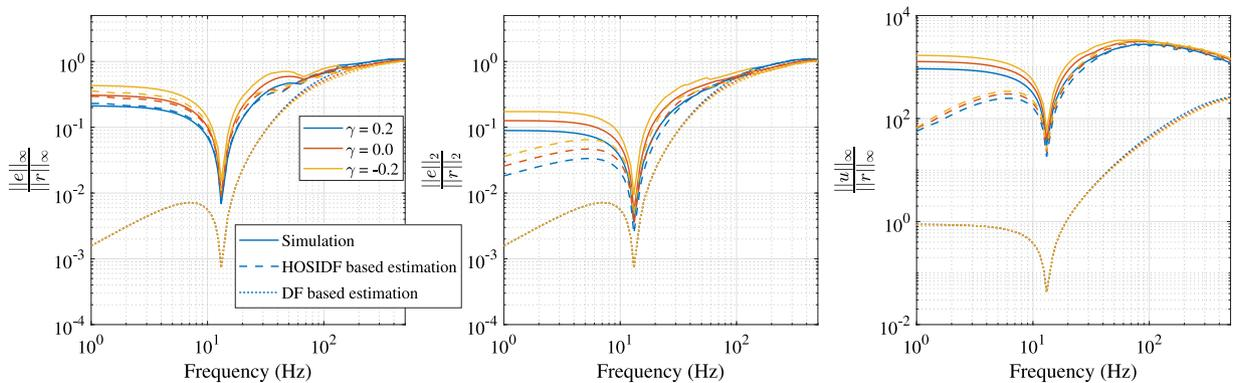
Fig. 16. Sensitivity plot  $\frac{\|e\|_\infty}{\|r\|_\infty}$ ,  $\frac{\|e\|_2}{\|r\|_2}$  along with control sensitivity  $\frac{\|u_R\|_\infty}{\|r\|_\infty}$  plotted for the three  $\mathcal{R}_{C_1}$  controller (refer (45)) based RCS.
