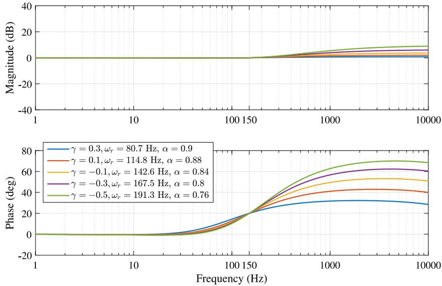
Fig. 2. Describing function of multiple CgLp elements designed to provide  $20^\circ$  phase compensation at 150 Hz. Slight deviation from unity gain is seen due to the nonlinear frequency behaviour of the GFORE.
