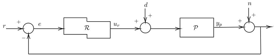
Fig. 1. Reset Control System with linear plant  $\mathcal{P}$  and reset feedback controller  $\mathcal{R}$  with reference  $r$ , process noise  $d$  and measurement noise  $n$ .
