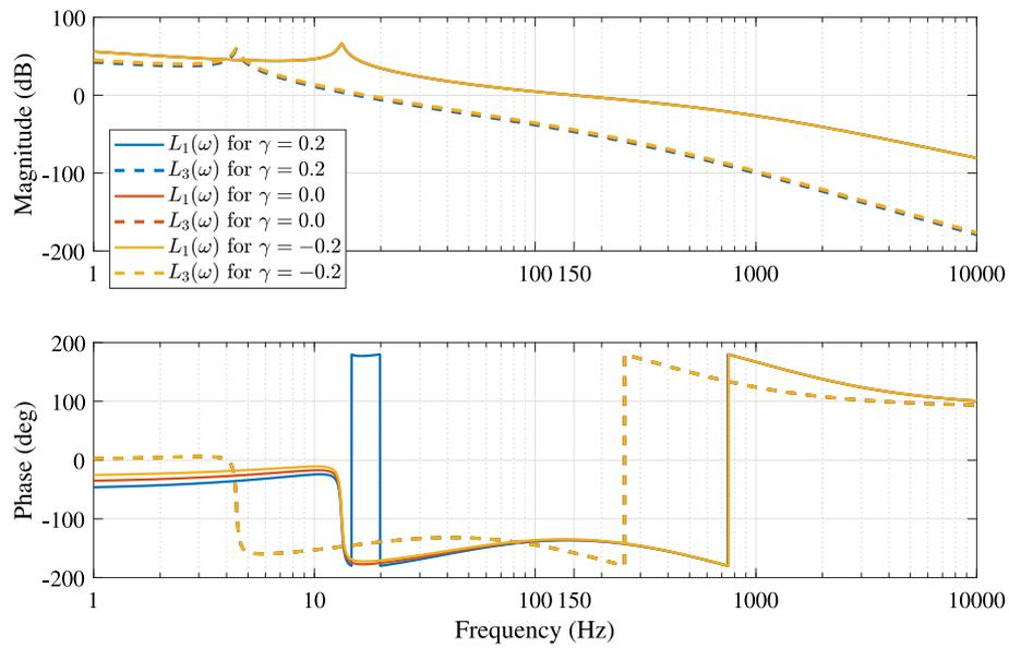
Fig. 13.  $L_1(\omega)$  and  $L_3(\omega)$  plots for three  $\mathcal{R}_{PCI}$  controller (refer (46)) based RCS with  $\gamma = \{0.2, 0.0, -0.2\}$ .
