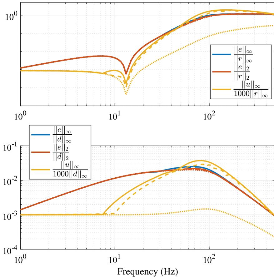
Fig. 20. Sensitivity plot  $\frac{\|e\|_\infty}{\|r\|_\infty}$ ,  $\frac{\|e\|_2}{\|r\|_2}$ , control sensitivity  $\frac{\|u_R\|_\infty}{\|r\|_\infty}$ , process sensitivity  $\frac{\|e\|_\infty}{\|d\|_\infty}$ ,  $\frac{\|e\|_2}{\|d\|_2}$  and control sensitivity to disturbance  $\frac{\|u_R\|_\infty}{\|d\|_\infty}$  plotted for  $C_{04}$  based RCS. Solid lines - 'Simulation', Dashed lines - 'HOSIDF based prediction', 'Dotted lines' - DF based prediction'.
