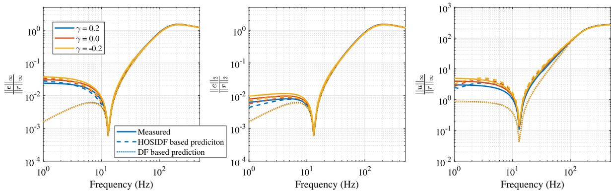
Fig. 18. Sensitivity plot  $\frac{\|e\|_\infty}{\|r\|_\infty}$ ,  $\frac{\|e\|_2}{\|r\|_2}$  along with control sensitivity  $\frac{\|u_R\|_\infty}{\|r\|_\infty}$  plotted for the three  $\mathcal{R}_{PC1}$  controller (refer (46)) based  $\mathcal{RCS}$ .
