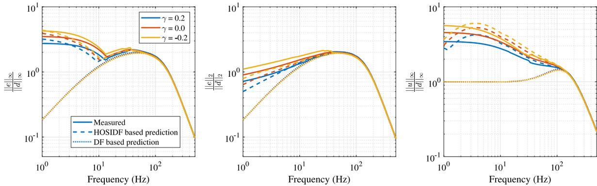
Fig. 19. Process sensitivity plot  $\frac{\|e\|_\infty}{\|d\|_\infty}$ ,  $\frac{\|e\|_2}{\|d\|_2}$  along with control sensitivity to disturbance  $\frac{\|u_R\|_\infty}{\|d\|_\infty}$  plotted for the three  $\mathcal{R}_{PC1}$  controller (refer (46)) based  $\mathcal{RCS}$ .
