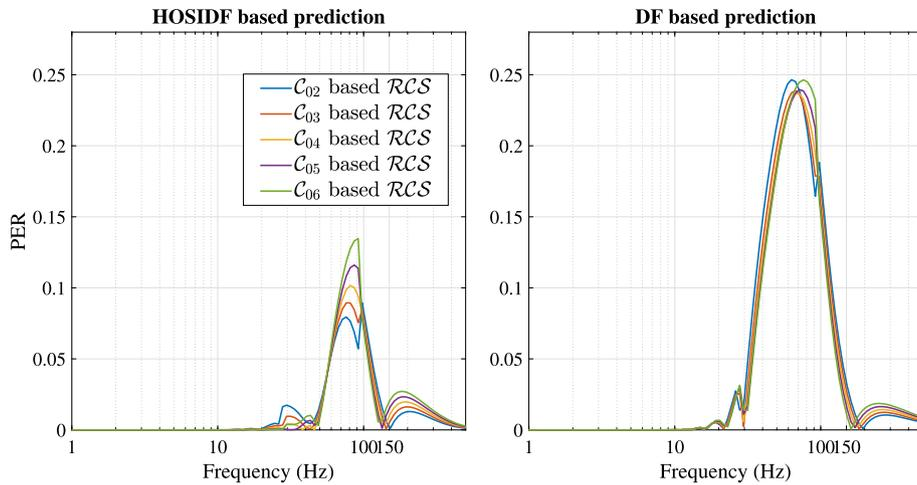
Fig. 21. Prediction error ratio plots of  $C_{02}$  to  $C_{06}$  based systems for input  $r$  based on  $L^\infty$  norm for the existing DF based and novel HOSIDF based methods. All systems have same  $|L_1|$  and PM.
