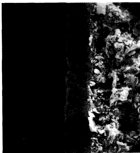
5 \mu\text{m} Fig. 12. Side view of SiC deposited on a graphite plate
