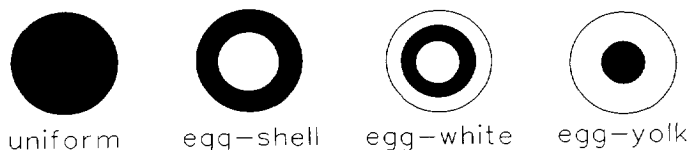
Fig. 1. Activity profiles in catalyst pellets. The black areas represent the place of highest concentration of the active phase
