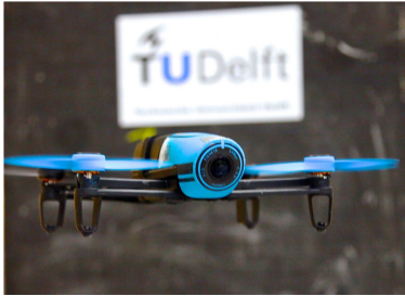
Figure 3. The Parrot Bebop 1 is used as experiment platform. The software is replaced by the Paparazzi UAV open-source autopilot project. Image from [12].
