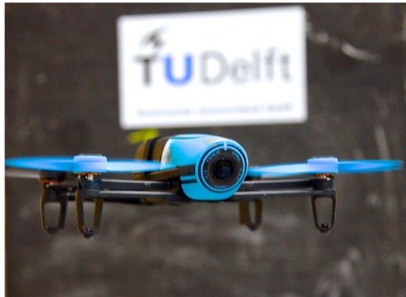
Figure 5.1: The Parrot Bebop 1 is used as experiment platform. The software is replaced by the Paparazzi UAV open-source autopilot project. Image from [7].
