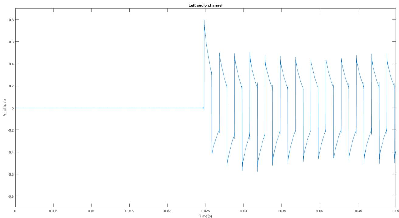
Figure 4.10: This figure shows the safe delay that the synchronization setup uses to start the audio recording synchronous with the ultrasound recording: it makes sure the audio is first running, then triggers the Zonare. The signal in the plot is not the actual signal, but a scaled down and capacitively coupled signal to meet the audio recorder maximum voltage levels.
