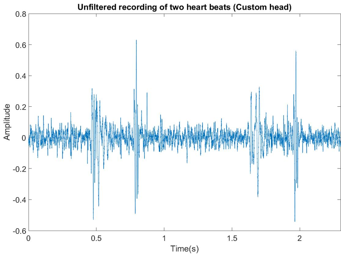
Figure 4.6: This figure shows the time domain of two heart beats recorded with the custom stethoscope head. Based on this data, also the dynamic range is determined. This signal is not yet filtered or corrected for the recorder response.
