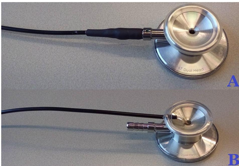
Figure 3.1: A: The TOM-1545P-R microphone is built into the metal tube connector of the analog stethoscope head. B: The TOM-1545P-R microphone is built into the central tube of the analog stethoscope head.
