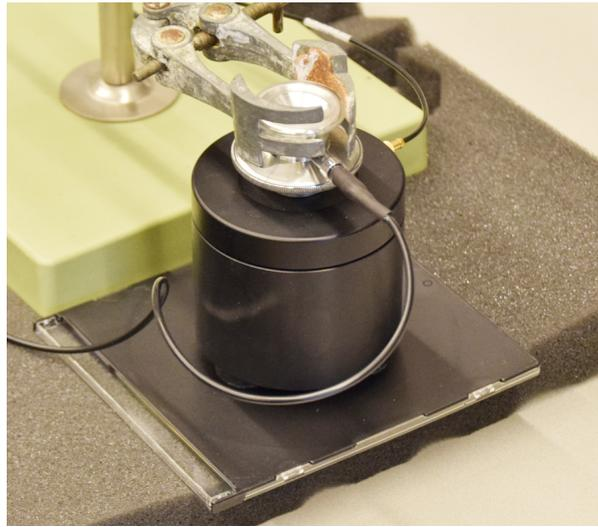
Figure 4.1: This figure shows the vibration generator measurement setup. The vibration generator is right below the stethoscope head membrane, the stethoscope head is placed inside a clamp that is connected to a stand. The foam (used in some test) is also visible.
