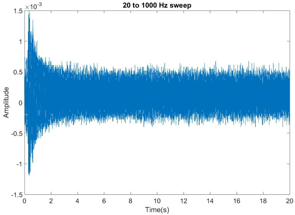
Figure 4.4: Time sweep from 20 to 1000 Hz using the mechanical vibration generator. The plot shows amplitude versus time. The frequency linearly increases from 20 to 1000 Hz in a time span of 20 seconds.
