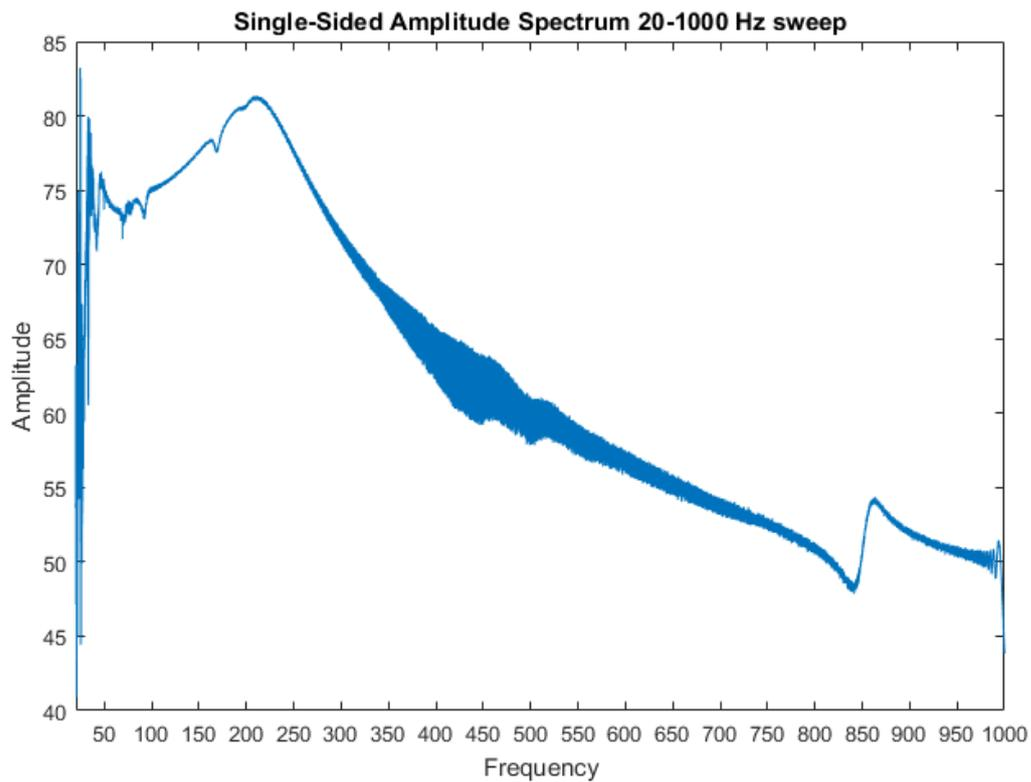
Figure 4.5: Frequency spectrum of the 20-1000 Hz sweep using the setup in figure 4.1. The plot shows amplitude versus frequency. A low-pass filter characteristic is visible.
