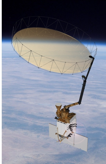
Figure 4: A depiction of the Northrop Grumman AstroMesh antenna, positioned on the NASA Jet Propulsion Laboratory Soil Moisture Active/Passive mission, launched in 2015. Its technology was trusted by JPL in fulfilling a goal presented in the first Earth Science Decadal Survey. 12
