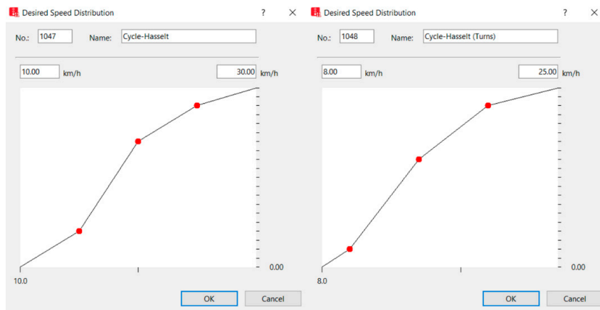
Figure 4. Implemented speed distributions for cyclists for normal routes (left) and turns (right).
