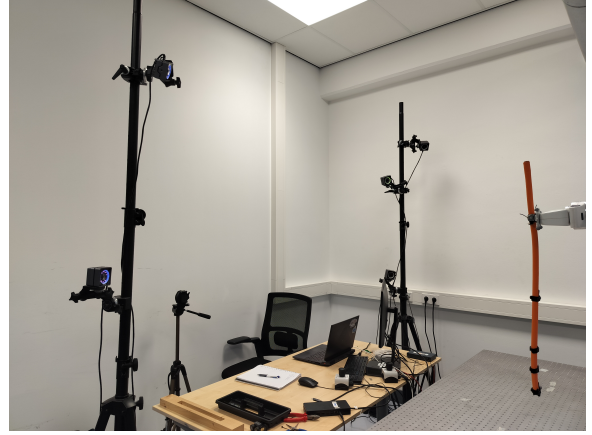
(b) Optical tracking setup (OptiTrack) to record marker positions
