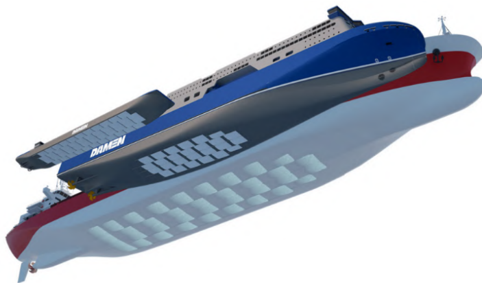
Figure 2.5: The Damen Air Cavity System (DACS) for different ship types, (Damen Shipyards Group, 2023).
