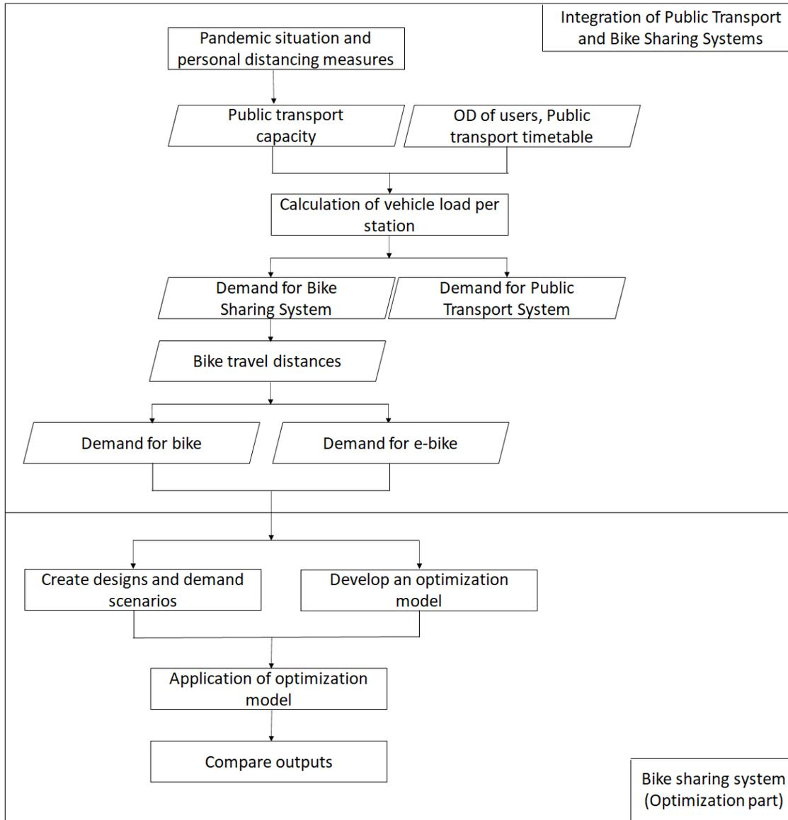
**FIGURE 2:** This is the modeling framework. It shows the various steps of the process and their sequence. The rectangles represent a process or a state, while parallelograms are used for input or output operation. The arrows connect the symbols and indicate the flow of process and information.
