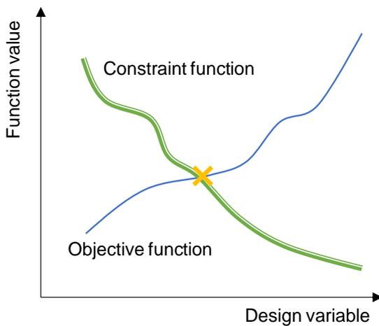
Figure 38 - Example simple search space: only one minimum is present.
