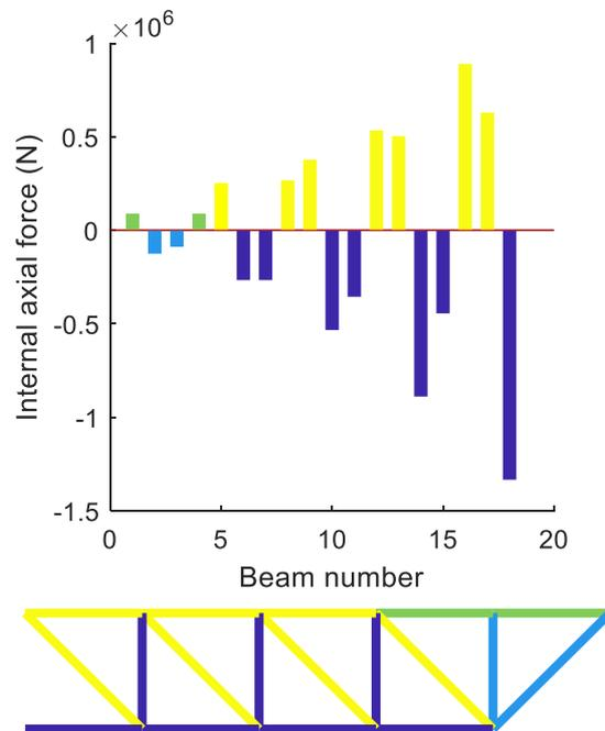
Figure 22 - Axial force distribution AF+W and weakening of two least-loaded members in each group.
