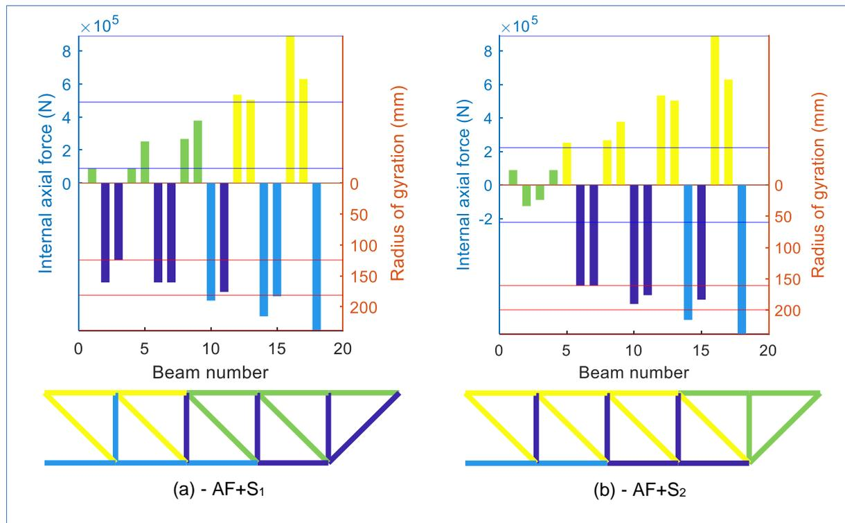
Figure 21 - Comparison axial force and radius of gyration distribution, and grouping procedures AF+S.
