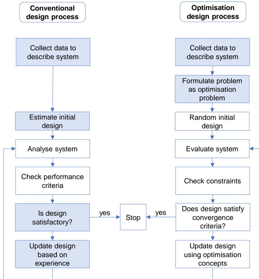
Figure 4 - Conventional design process versus optimisation design process: the repetitive tasks are automated. Blue shading shows the need for experience of an engineer. Adaptation of original figure in literature (Arora 2017).
