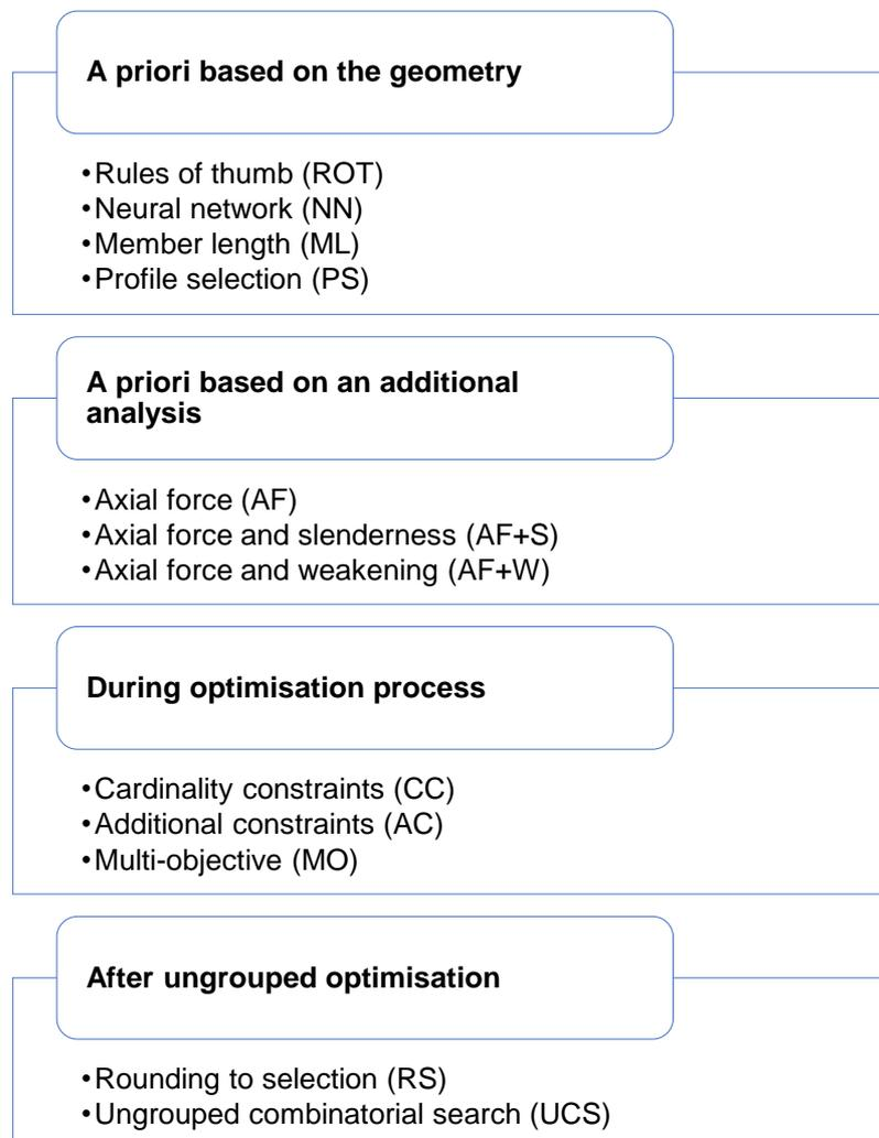
Figure 15 - Overview grouping methods which categorisation on moment at which the groups are formed.
