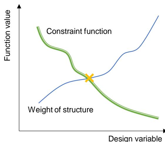
Figure 6 - Example search space weight optimisation. Yellow cross indicates global optimum, no local optima are present.
