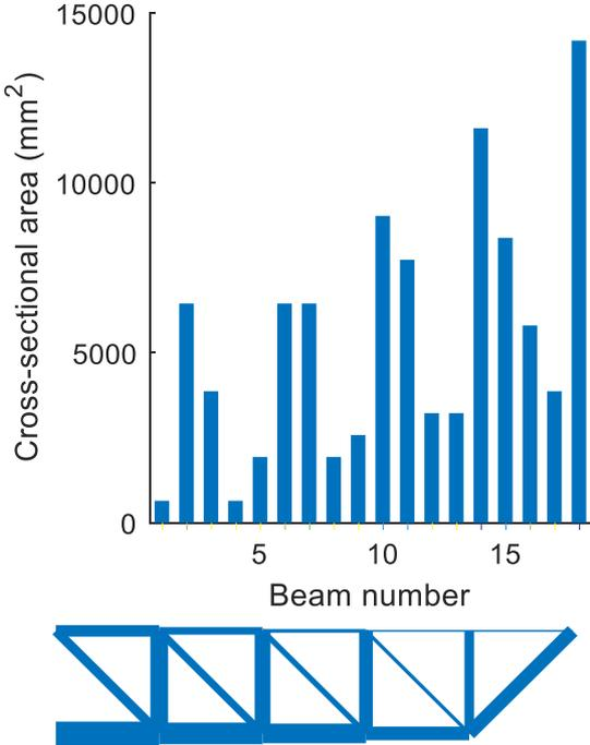
Figure 28 - Solution cross-sectional area ungrouped solution, no grouping is shown as no decisive guidelines are available to do so.
