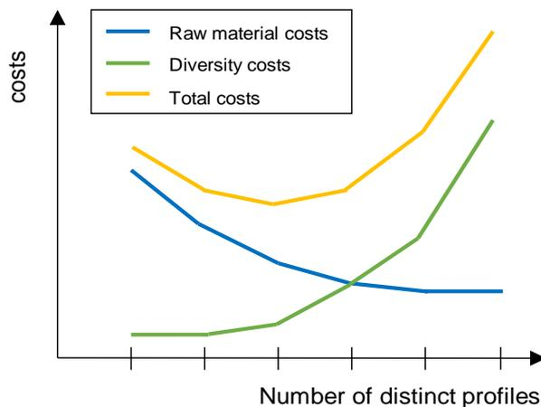
Figure 10 - Comparison of costs, adaptation of original figure (Gutkowski 1997). Total costs are sum of diversity and raw material costs, which creates an optimum for a limited number of distinct profiles.
