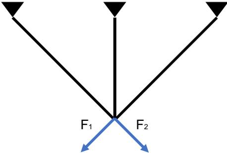
Figure 2 – Three-bar truss Schmit subjected to two independent load cases. Adaptation of original figure in literature (Vanderplaats 1993).
