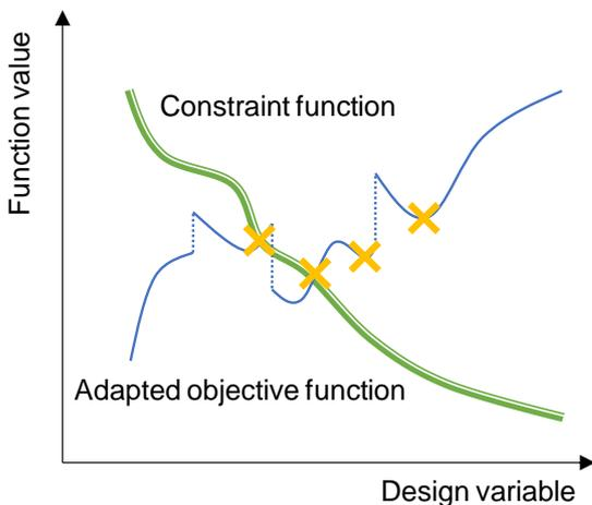
Figure 41 - Example altered objective function in search space MO: creation of additional local optima.
