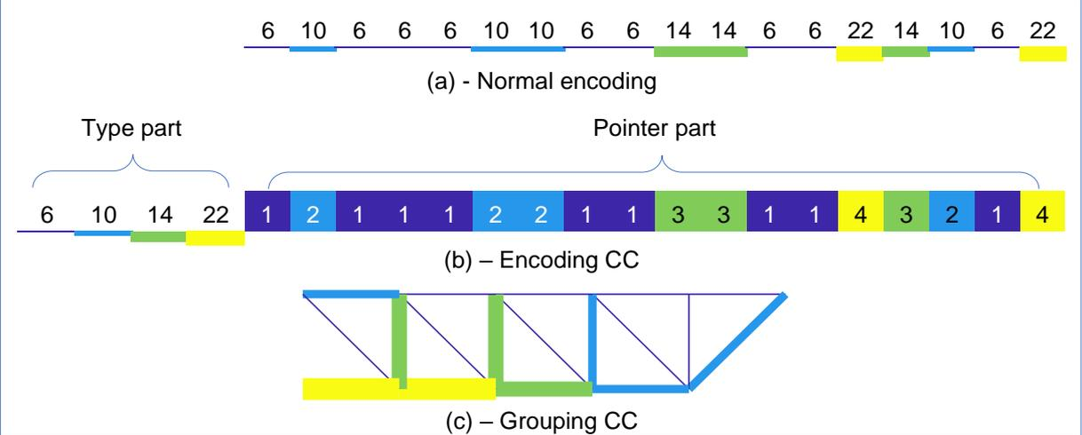
Figure 24 – Example normal encoding and encoding CC for same grouping.
