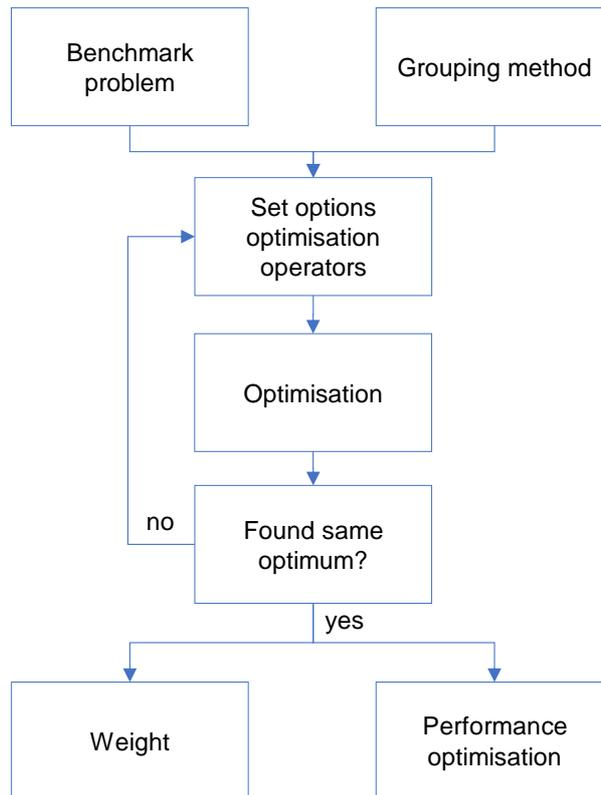
Figure 44 – Flow chart numerical experiments. For every grouping method and benchmark problem, the optimisation parameters are altered.
