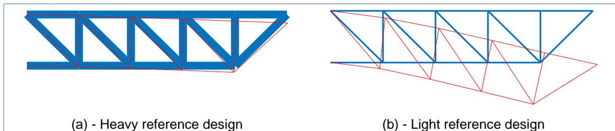
Figure 32 – Example influence reference design. The global displacement is strongly influences by the references design, thereby influence the result of the fully stressed design.
