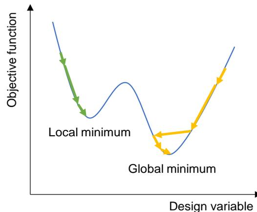
Figure 5 - Example of local and global minima, and iterative search by search methods. Individual searches can find a different minimum.
