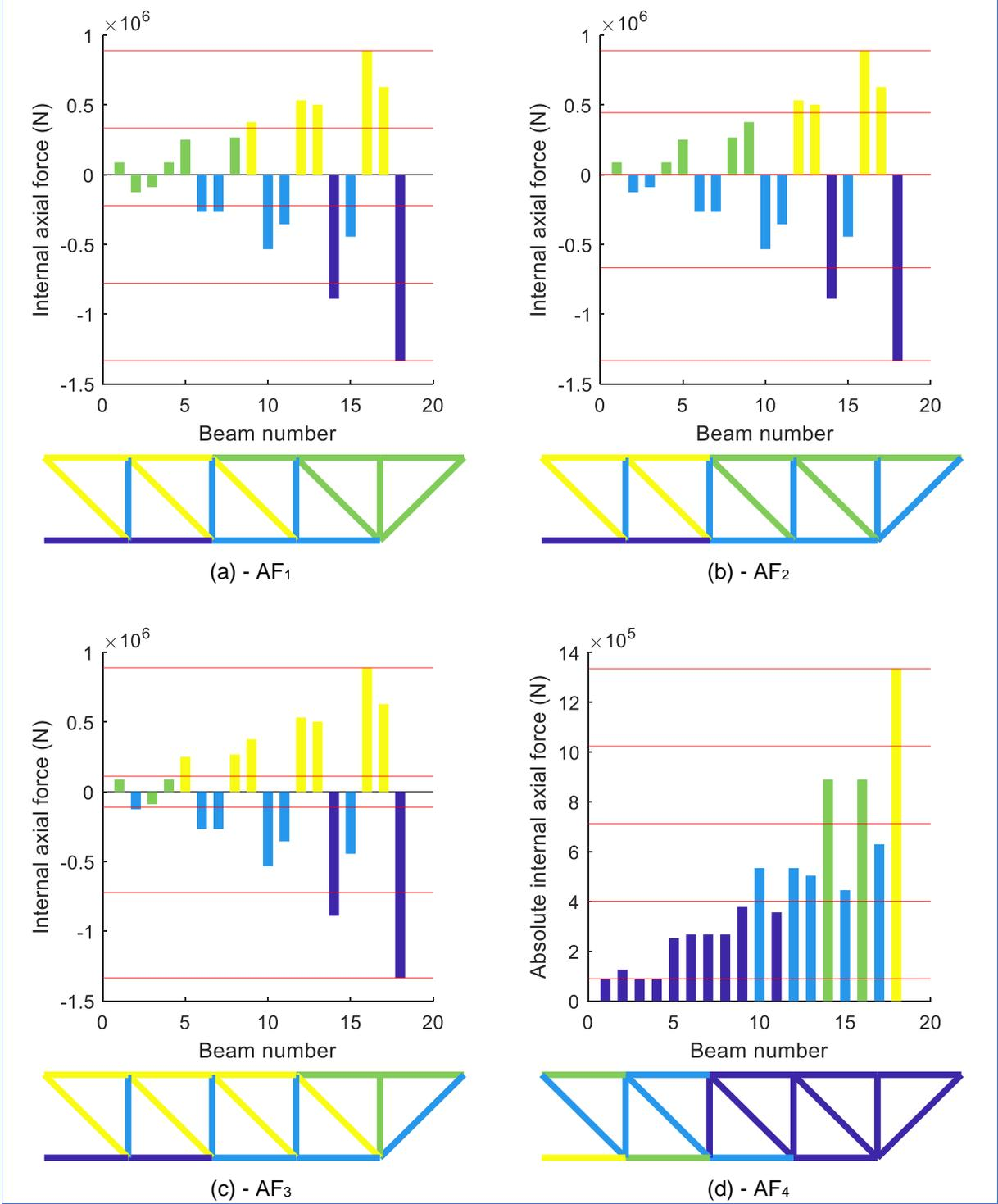
Figure 20 - Comparison axial force distribution and grouping procedures AF.
