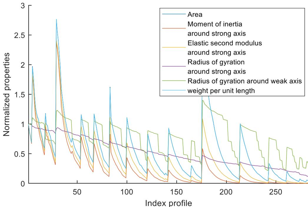
Figure 99 – Order of properties of steel profiles
