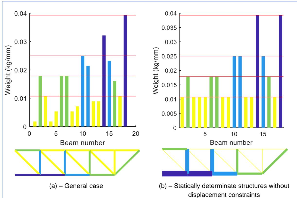
Figure 33 - Example weight distribution fully stressed design FSCS.
