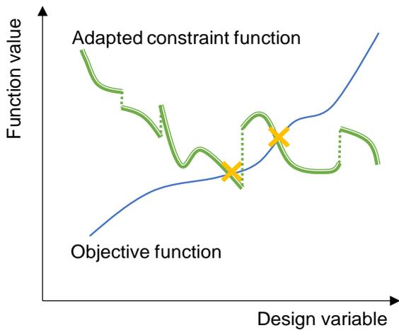
Figure 40 - Example altered constraint function in search space AC: creation of additional local optima.
