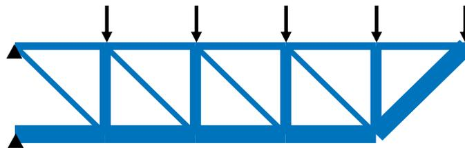
Figure 9 – Example minimum cost design: few unique profiles.
