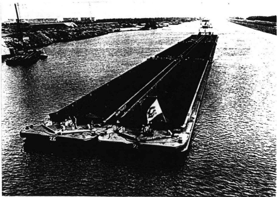
Fig. 2.5 Pushing unit 3 x 2 loaded length 229.5 m, width 23.6 m, draught 3.0 m
